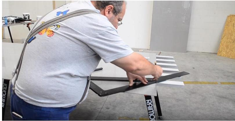
Once the cut has been made, it must be “opened” (meaning that the parts of the glass layer divided by the cut must be completely separated). This operation can be performed by hand or by using glass pliers.
