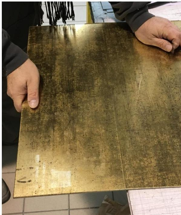
Turn the slab upside-down and perform the same operation on the other side of the slab. Make sure that the trajectory along which the second cut is performed perfectly matches the position of the trajectory along which the first cut had been performed. Even in this case, “open” the cut following the instructions provided above.
