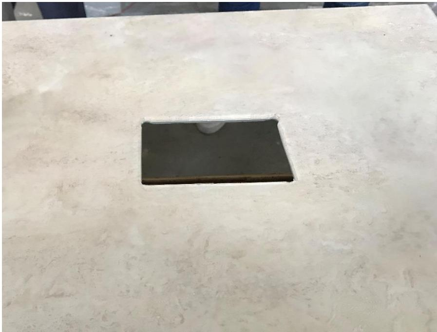
Even when making a slot or notch it will be necessary to polish the edges that have been cut. This operation can be accomplished by using an angle grinder as the one described above or, in case the slot is too small making the angle grinder impossible to use, by polishing the edges using some abrasive sandpaper.
