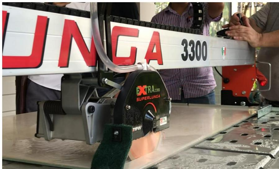
Keep the blade of the saw constantly wet in order to avoid that the heat caused by the friction produced by the saw that cuts the slab damages the glass.
