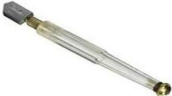
Being Vetrone made of two glass slabs, the manual cut must be performed on one side of the slab and then on the other. Perform the cut by dragging the glass cutter along the desired trajectory of the cut. Use a geometric square for glass in order to obtain a straight cut. In case of a particularly long cut, lubricate the trajectory of the cut by covering it in oil for glass (like that contained inside the glass cutter) so that performing the cut will result more fluid and overall easier.
